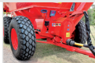
- Monoblock chassis. - Heavy-duty front and rear axles. - Self supporting towbar.
