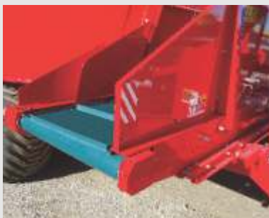
Hydraulically operated right-side discharge PVC belt conveyor.
