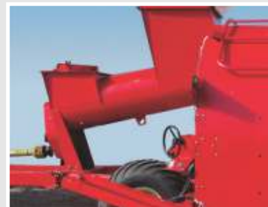
500 mm diameter auger for big loading capacity.
