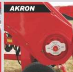
Roll transmission achieved through a sturdy reduction gearbox and only one chain.
