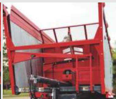
Exclusive push-off compression and discharge system. Towbar with height adjustment.
