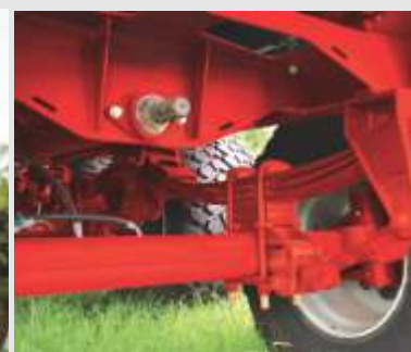
Steering axles fitted with lock sensors. Akron chassis.
